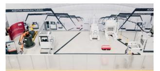
The built-up pilot plant of the NextGenAM project for automated additive manufacturing in detail, from left to right: band saw, Kuka robot, background: three-dimensional optical measurement system, setup station, unpacking station, forefront: automated guided vehicle (AGV), EOS M 400-4, not pictured: IPM M Powder Station L from EOS (Source: EOS).
